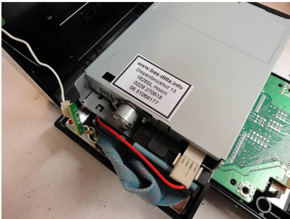
The new disk drive is installed and the cables are connected.
